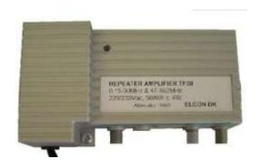
TF30 is a broadband repeater amplifier for AM, FM and TV reception to be used in CAS systems with 20 outlets and up, in connection with our usual head- end amplifier to cancel the cable losses. It has a built- in equalizer  $0-10~\mathrm{dB}$  for the right output level.
